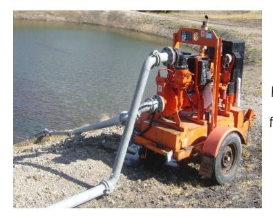
The 4" x 3" HL80, a High Head Trash Pump, supplied high pressure clean water back into the pond through 4" Bauer pipe and fire hoses to break up and ease the movement of sludge from one pond to the other.
