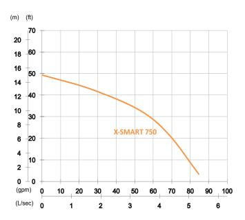
Shaft Speed: 3450 rpm Outlet: 50mm, 2in
