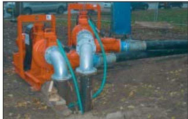
Two Godwin CD225M electric drive Dri-Prime pumps on rent in Holland.
